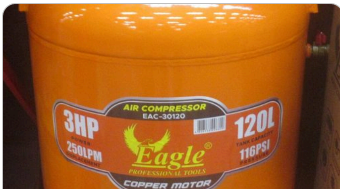
Air receiver — stores air, smooths demand peaks and separates moisture
