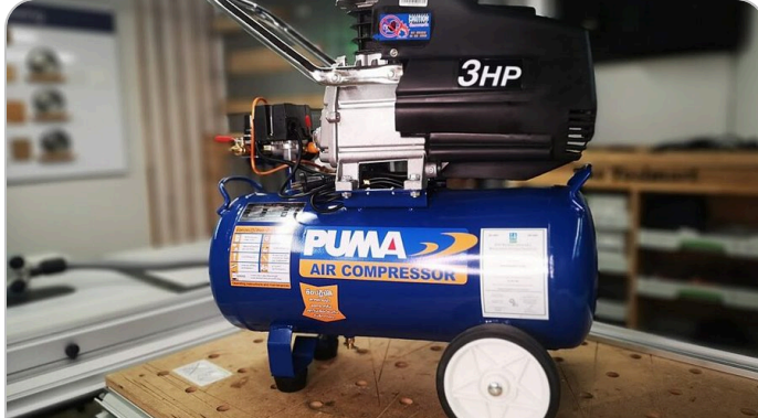
Small reciprocating (piston) air compressor with its receiver
