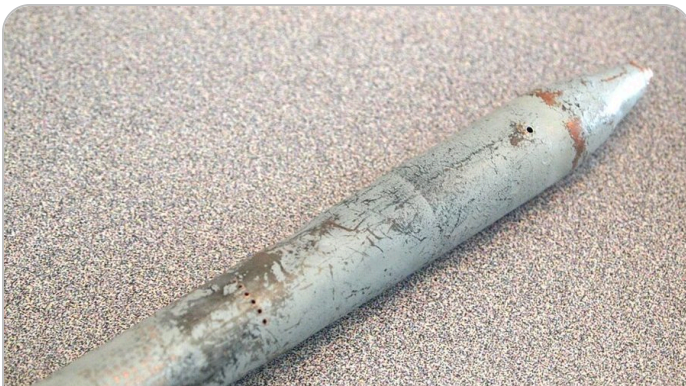
Pitot-static tube — measures velocity pressure for duct flow
