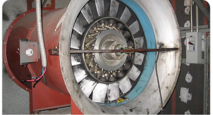
Axial-flow fan — air enters and leaves along the shaft with no change of direction
